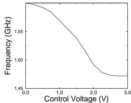
Figure 3: Output frequency versus control voltage
