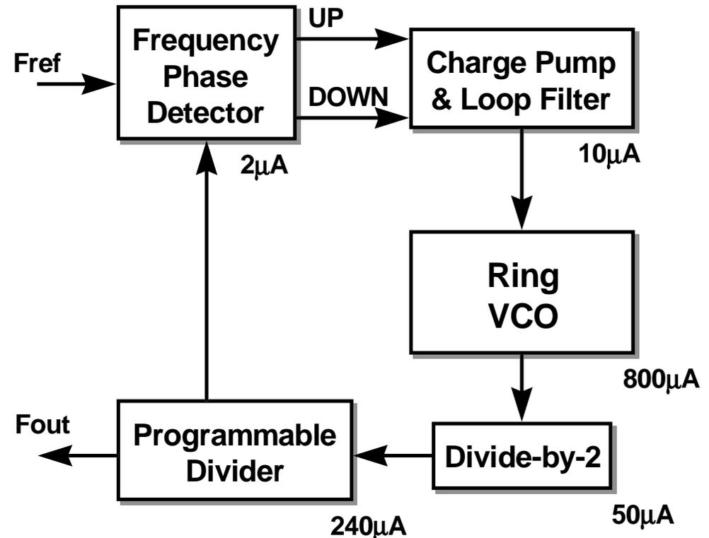
Power budget for a typical CMOS PLL frequency synthesizer used in microprocessor clock generation<sup>1</sup>.
