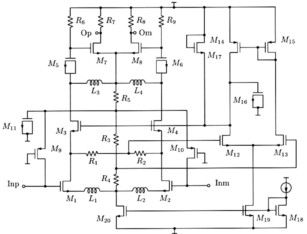
22-3-2: LNA circuit schematic.
