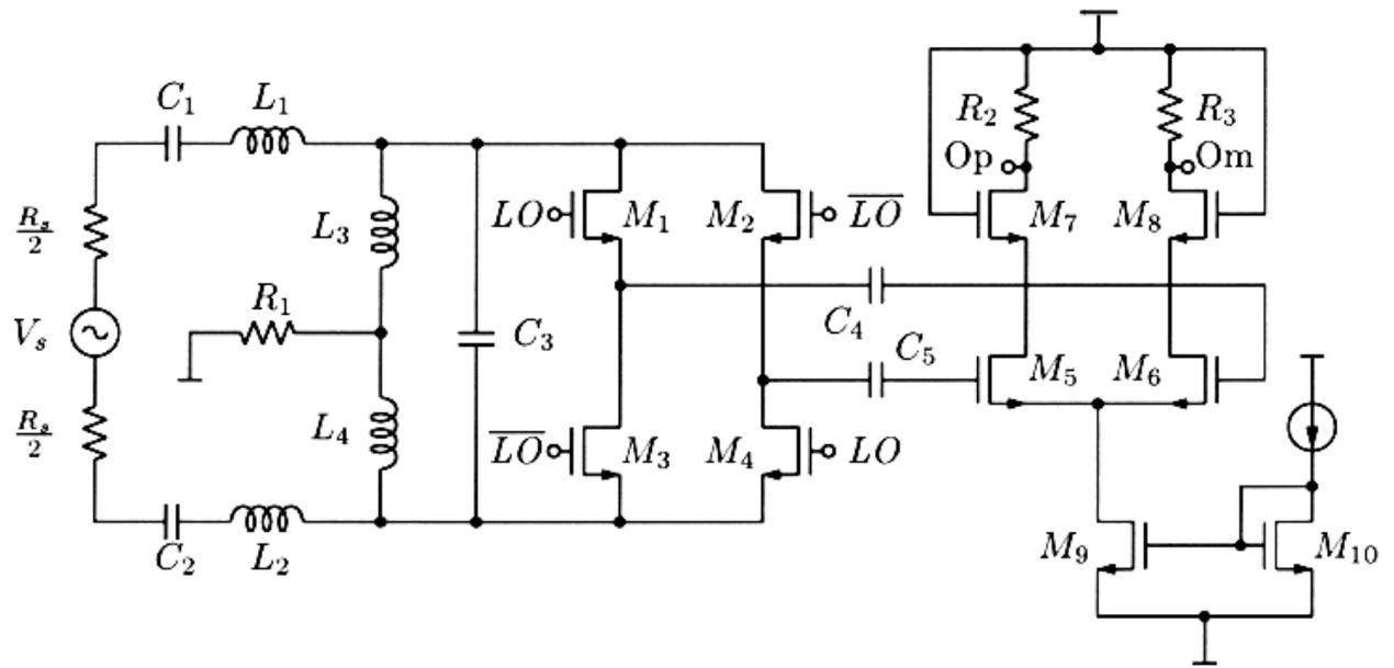
22-3-4: Schematic of mixer circuit with test buffer.
