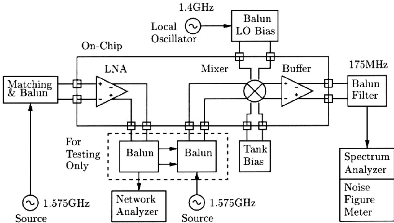
22-3-1: Block diagram of the GPS front-end test setup.
